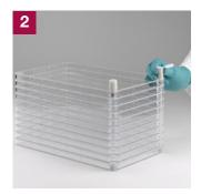
Remove vent closure and replace with white Tyvek $^{\text{M}}$  adaptor cap.
