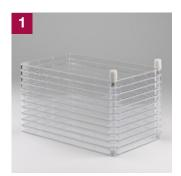
Unpack the Nunc Cell Factory system and place it in a laminar air flow cabinet in order to work in sterile conditions.
