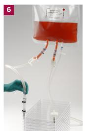
Connect the male MPC from the bag to the female MPC on the Cell Factory system.
