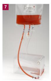
Turn the Cell Factory system on side with air filter up. Open clamp to start filling. Medium will level out between the trays during filling.
