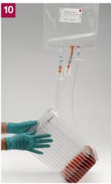
Turn Cell Factory system into incubation position. The Cell Factory system is now ready for incubation.
