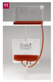
To empty the Cell Factory system, place it above the media and release clamp.
