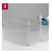
Immediately insert pre-sterilized air filter into the open white filter adaptor cap.
