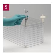
Remove vent closure before attaching the tubing set with the female MPC to the open port.
