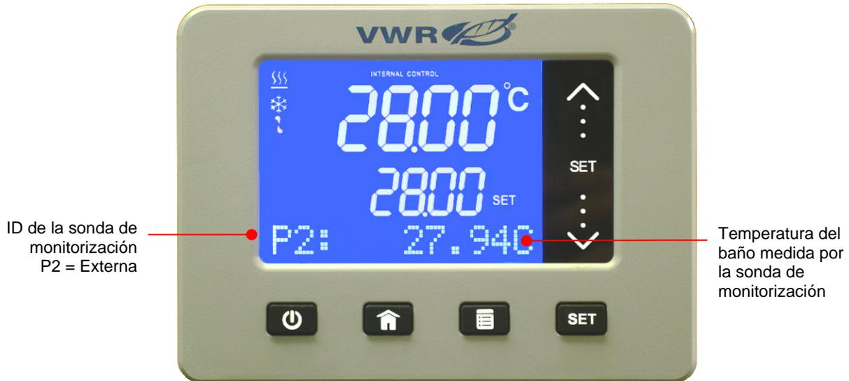
*Control interno (P1) – sonda externa (P2) conectada*
