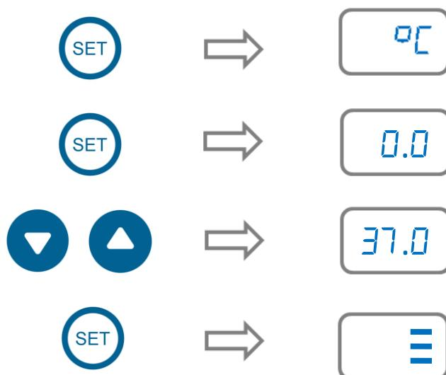
Once the control temperature is entered the bath shows a scrolling bar display indicating the bath is heating. When the bath is within 1°C of the control temperature this will change to displaying the actual water temperature in the bath.
