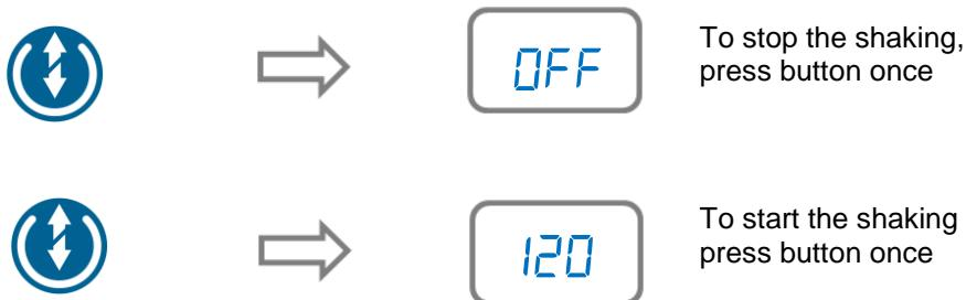
The shaking will start at the speed previously set using the **rpm** button. If no speed has been set then the display will show **OFF** when **start** is pressed.
